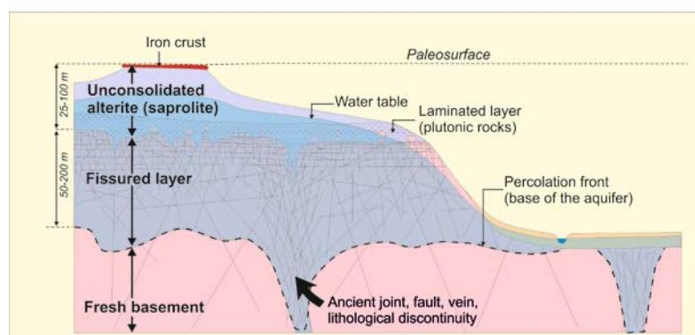
Figure 1 – Structure of a lateritic profile partially eroded by the present topography
